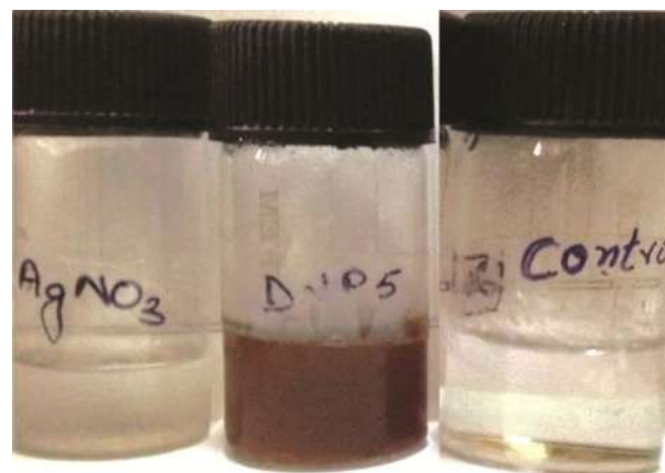
Fig. 2 — Extracellular synthesis of silver nanoparticles
